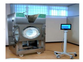
Figure 10. The setup of the industrial scale microwave extractor MAC 75/Milestone Technologies.
